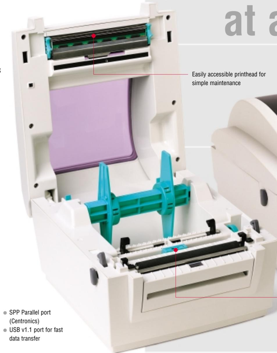
Easily accessible printhead for simple maintenance
